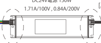
[WKLZ240-6R3H] DC24V電源 150W 1.71A/100V, 0.84A/200V
